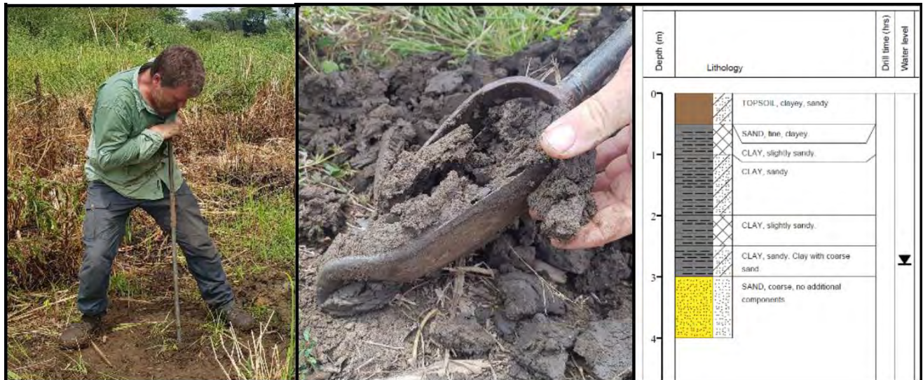
Figure 2 From left to right: Augering kit in use ; Soil sample analysis ; Test drill report Alakas
